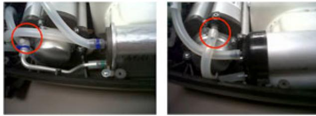
Figure 5--ATF Outlet Location for Tubing Connection
